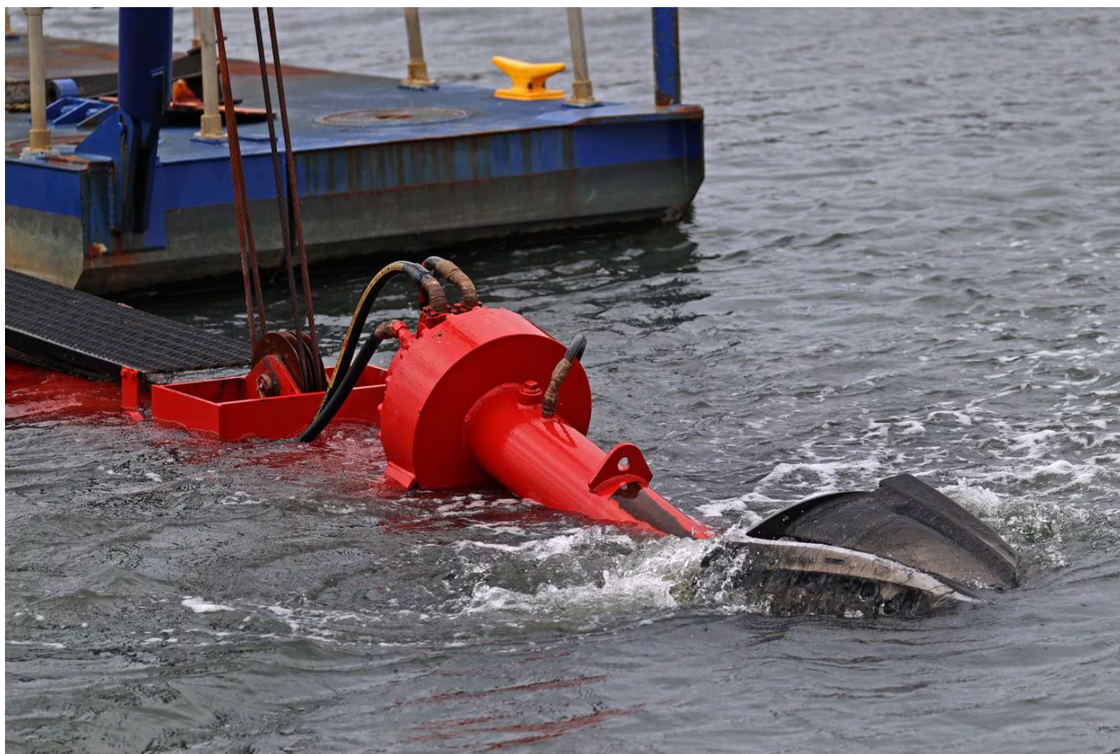
A view of a cutter head dredge being used by the entrance of Allen Harbor in Harwich. DAVID L. RYAN/GLOBE STAFF
